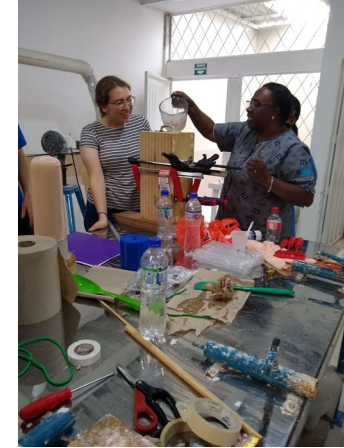
Pouring soft silicone into mold
